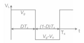
Fig: 8. Inductor voltage waveform
