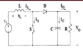
Fig: 4. Circuit diagram of boost converter
