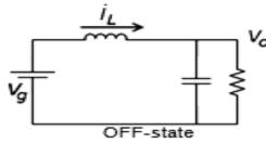
Fig: 5. The OFF state diagram of the boost converter
