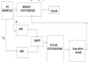
Fig: 1. Block Diagram of Photovoltaic system using boost converter with MPPT
