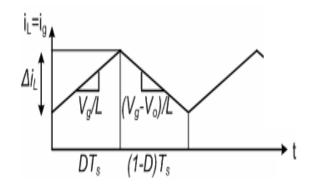
Fig: 7. Inductor current waveform
