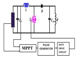
Fig: 2. Circuit Diagram of Photovoltaic system using boost converter with MPPT
