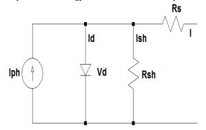
Fig: 3. Basic equivalent circuit of solar cell
