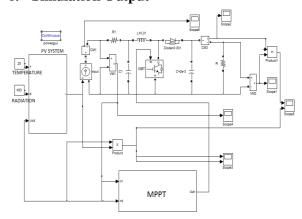
Fig: 9. Stepup Boost Converter for PV System
